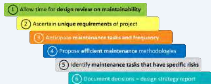
Figure 1: Engaging stakeholders across the value chain at design stage to ensure maintenance considerations are accounted for.
