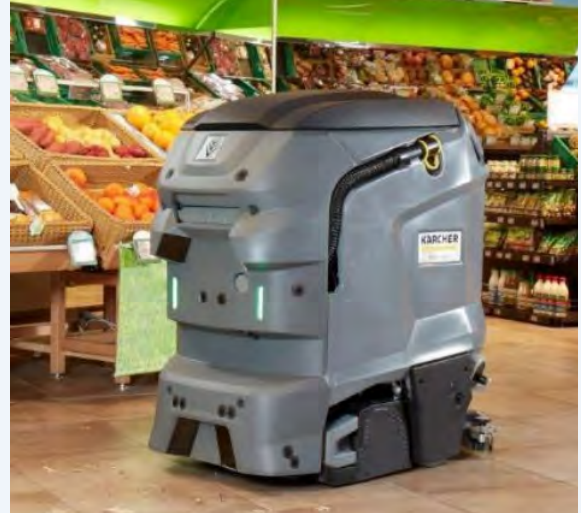
Figure 5: Adoption of robots cleaning machines requires several upstream considerations such as minimal floor level differences and interoperability with the building infrastructure, e.g. lifts and automated doors.
